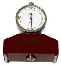
The mesh tension for each frame is provided by the frame manufacturer in five locations. When reviewing the measurement<del>s</del> data for about 3000 meshed frames, the results are very impressive and consistent. The Mesh Tension range is 30-36 Ncm with a nominal of 33 Ncm.
